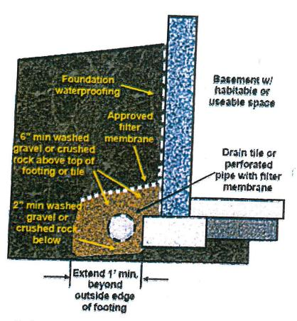
Drains must discharge by gravity or mechanical means to an approved drainage system
