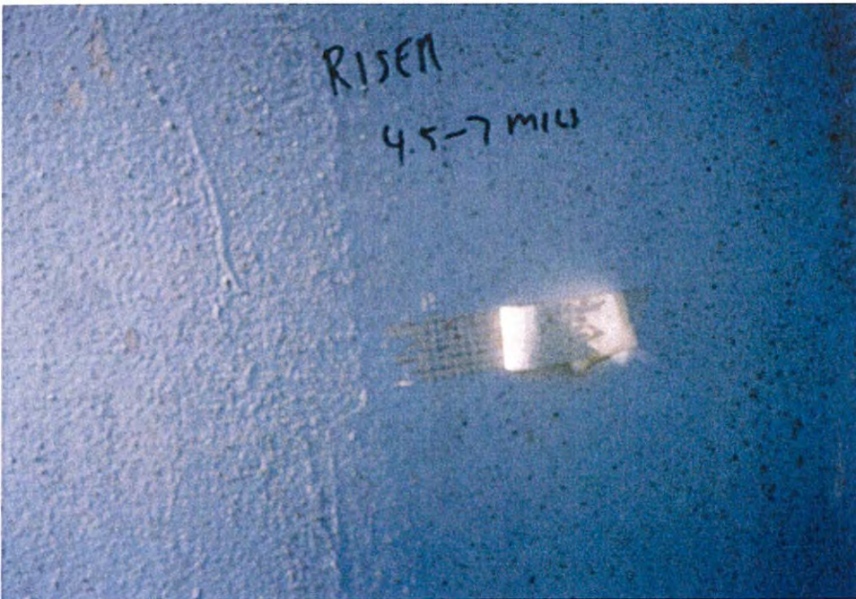
26. Coating thickness measurements and coating adhesion test on exterior riser.
