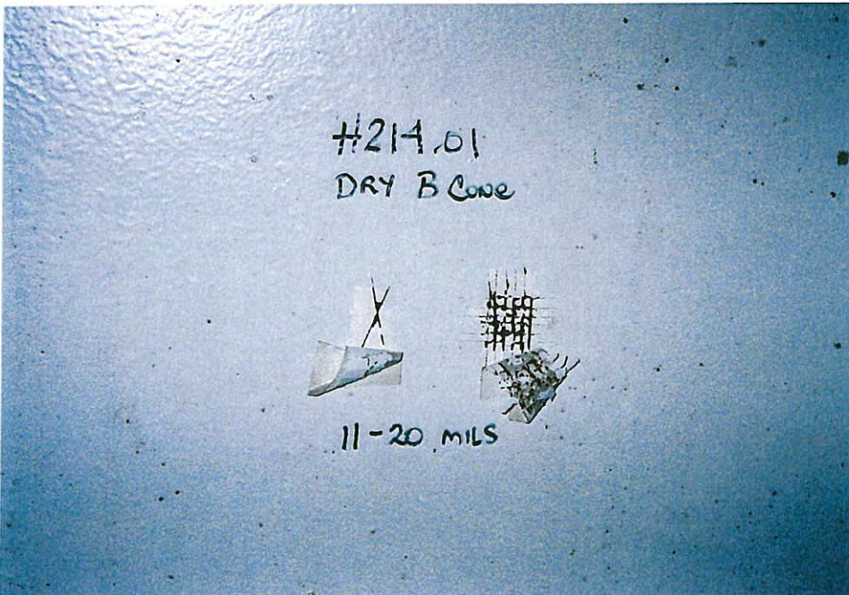
54. Coating thickness measurements and coating adhesion tests on in dry base cone.
